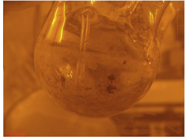
Fig. 11. Photograph of sludge generated from irradiated fuel.
