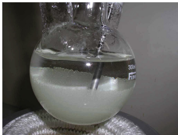
Fig. 1. Photograph of sludge generated from non-radioactive reagents.
